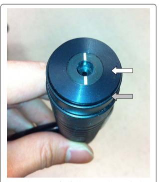
**Figure 3 Cutometer probe.** The Cutometer probe viewed end on. The white arrow shows the spring mounted contact surface which contains the 6 mm aperture. The grey arrow shows the rigid external shell that is held by the operator.
