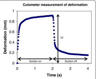
**Figure 2 Cutometer loading and unloading curve.** Typical deformation curve of skin under one cycle of loading and unloading. The Cutometer measures deformation of skin in millimeters as a function of time in seconds. Here, 45 kPa of suction was applied for 2 seconds, followed by no suction for 2 seconds. Uf is labeled and represents the maximal amount of skin deformation due to the suction load.
